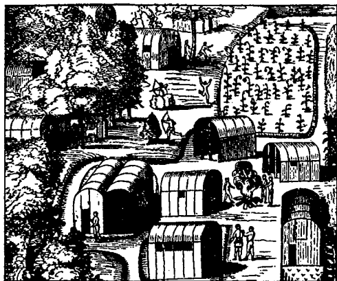
FRAME CONSTRUCTION is indigenous to the U. S. When Capt. John Smith landed in Virginia he found the Indians living in houses of light wood frame covered by sheets of bark and skin; but no glass.
